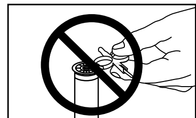
INCORRECT WAY TO ADJUST ARC
